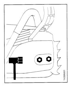
You can run chains of different pitches on this chainsaw - depending on the chain sprocket (see "Specifications")
