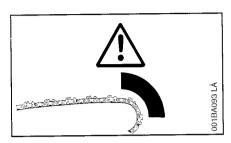
powerful force used to cut wood can be reversed (and work against the operator). If the rotating chain is suddenly stopped by contact with any solid object like a log or branch or is pinched, the reactive forces may occur instantly. These reactive forces may result in loss of control which may, in turn, cause serious or fatal injury. An understanding of the causes of these reactive forces may helpyou avoid loss of control.
