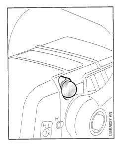
Only machines with easy start system: Prime the fuel system:
