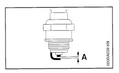
Wrong fuel mix (too much engine oil in the gasoline), a dirty air filter and unfavorable running conditions (mostly at part throttle etc.) affect the condition of the spark plug. These factors cause deposits to form on the insulator nose which may result in trouble in operation.
