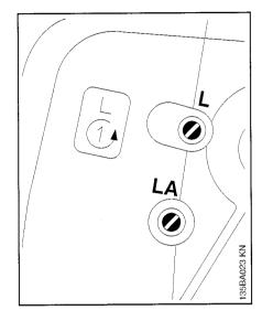
Engine stops while idling: 'L' screw must be one turn open.
