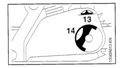
Place sprocket cover in position engage guide lugs in recesses in engine housing and check that the teeth of the adjusting wheel and tensioning gear mesh.
