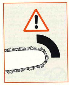
or branch or is pinched, the reactive forces may occur instantly. These reactive forces may result in loss of control which may, in turn, cause serious or fatal injury. An understanding of the causes of these reactive forces may help you avoid loss of control.
