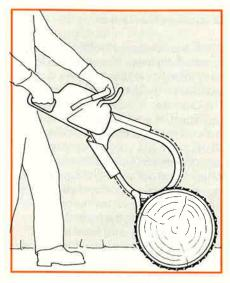
Warning! The risk of kickback is increased with a bow guide because of the increased kickback contact area. STIHL recommends the use of the STIHL Quickstop chain brake. Low kickback chain will not significantly reduce the risk of kickback injury when used on a bow guide.
