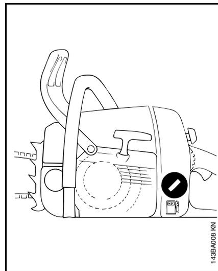
Before fueling, clean the fuel filler cap and the area around it to ensure that no dirt falls into the tank. Always thoroughly shake the mixture in the canister before fueling your machine.
