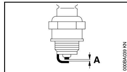
Wrong fuel mix (too much engine oil in the gasoline), a dirty air filter and unfavorable running conditions (mostly at part throttle etc.) affect the condition of the spark plug. These factors cause deposits to form on the insulator nose which may result in trouble in operation.
