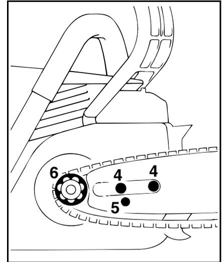
Fit the guide bar over the studs (4) - cutting edges on top of bar must point to right - and engage the peg of the tensioner slide in locating hole (5) - place the chain over sprocket (6) at the same time -
