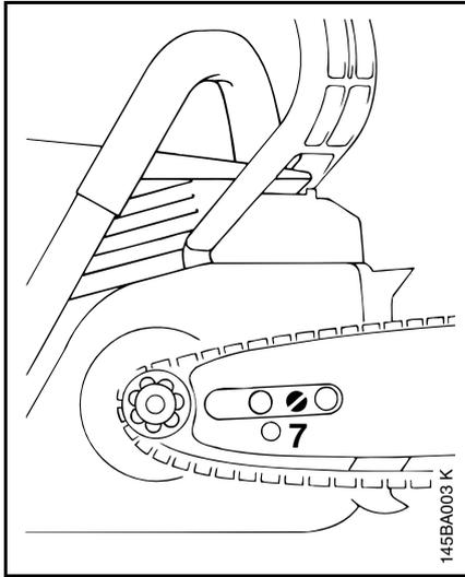
Now turn tensioning screw (7) clockwise until there is very little chain sag on the underside of the bar - and the drive link tangs are located in the bar groove.
