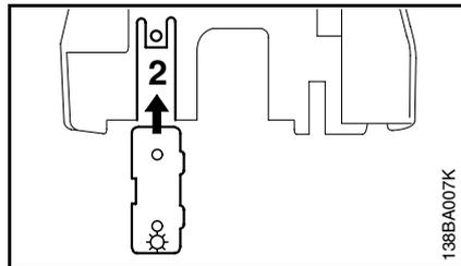
**Pry the shutter (1)** out of the carburetor box cover (summer position) and slide it into the slot **(2)** (winter position)
