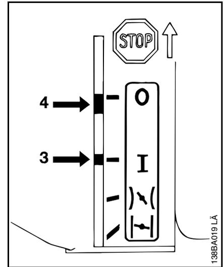
In the "Warm Start" position, continue cranking after engine begins to fire. As soon as the engine runs, **immediately** blip the throttle trigger so that the Master Control lever moves to "Run" - idling position - normal operating position (3).
