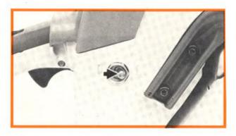
The handle heating system keeps the handle bar and pistol grip comfortably warm while the chain saw is being operated at extremely low outside temperatures.
