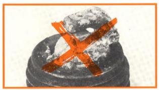
If the engine is down on power, difficult to start or runs poorly at idling speed, check the spark plug before looking any further. If the spark plug is dirty, clean it and check the electrode gap. Readjust if necessary; the correct gap is 0.5 mm (0.02 in). The spark plug should be replaced after about 100 operating hours or earlier if the electrodes are badly eroded.
