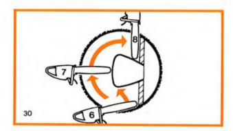
(ill.27). Next, align the saw in the direction in which the recess is to be cut.
