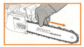
The Oilomatic chain is correctly tensioned when it fits snugly against the underside of the bar but can still be pulled easily along the bar by hand (with chain brake disengaged). Important: Wear protective gloves when performing this work.
