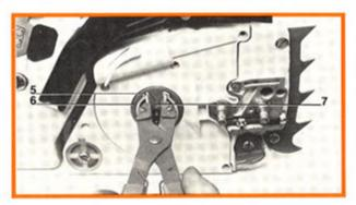
Remove the oil pump drive worm (8) from the pump shaft by turning it clockwise and pulling it at the same time. The chain sprocket (7) can now be pulled off the crankshaft together with the spur gear (9) and needle cage. The spur gear (9) can be prised off the chain sprocket (7) with the aid of two screwdrivers.
