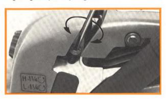
engine speed will be exceeded. This can cause engine damage, brought about by lack of lubrication and overheating in particular. Corrections to the setting of the high speed adjusting screw may be carried out only if an accurate tachometer is available to check the maximum engine speed of 13,000 r.p.m. (12,500 = 028 WB) (with bar and correctly tensioned chain).
