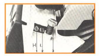
When the engine is tested at the factory the carburetor is set to obtain a slightly richer mixture to ensure that the cylinder bore and the bearings receive additional lubrication during the break-in period. This setting should be left as it is for the first three tank fillings. The high speed adjusting screw may then be turned no more than ½ turn clockwise (leaner mixture). Caution: The engine's maximum permissible rpm must not be exceeded!
