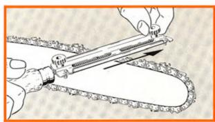
cutter heights will be uneven if the cutter lengths are different. If the cutters are not all the same height the chain will run roughly and eventually break.
