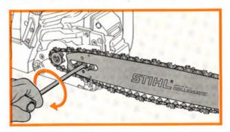
Hold the guide bar vertically with the nose upward and fit the Oilomatic chain on it, starting at the bar nose.
