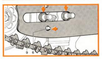
Pretensioning the chain (lateral chain tensioner)
