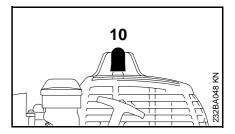
Move slide control or stop switch to STOP / O.
