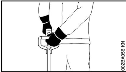
Always hold the trimmer firmly with both hands. Wrap your fingers tightly around the handles, keeping the handles cradled between your thumb and fore-finger. Keep your hands in this position, to have your trimmer under control at all times. Make sure your trimmer handles and grip are in good condition and free of moisture, pitch, oil or grease.
