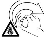
Unit vibrations can cause an improperly tightened fuel cap to loosen or come off and spill quantities of fuel.
