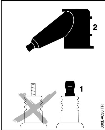
Always press spark plug boot (2) snugly onto spark plug terminal (1) of the proper size. (Note: If terminal has detachable SAE adapter nut, it must be attached.) A loose connection between spark plug terminal and ignition wire connector in the boot may create arcing that could ignite combustible fumes and cause a fire.
