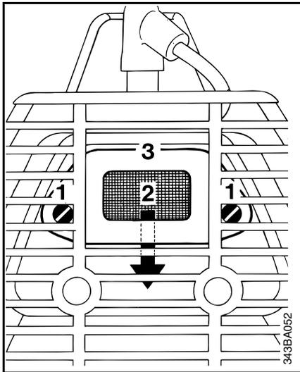
If the engine is low on power, check the spark arrester inside the muffler.
