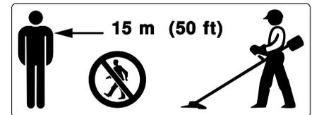
To reduce the risk of eye and other injury insure that bystanders are at least 50 feet (15 m) away. Stop the engine and cutting tool immediately if you are approached. Start and operate your trimmer without assistance. For specific starting instructions, see the appropriate section of your manual. Place the trimmer on firm ground or other solid surface in an open area. Maintain a good balance and secure footing.
