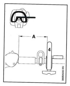
Align the loop handle (4) and move it to the most comfortable position.
