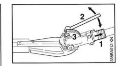
The angle of the cutter bar can be adjusted to 8 positions between 0° (straight) and 90° (right angle).
