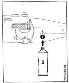
Use STIHL gear lubricant for hedge trimmers for lubrication of the **blade drive gear** (see "Special Accessories") after every 25 hours of operation.
