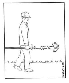
The scrub cutter may be carried only in a horizontal position. Grip the shaft in a manner that the machine is balanced horizontally. Keep the hot muffler away from your body and the cutting attachment behind you.
