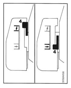
If engine is cold: Set the choke lever (4) to  $\mathcal{I}$
