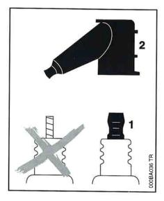
Fit a new spark plug after approx. 100 operating hours -
