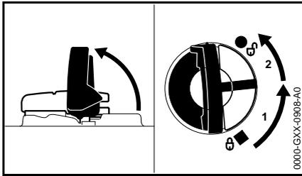
Flip up the lever and slowly turn left (1) to the vent position of the cap at about 1/8 turn where the cap is held in place by the thread. Once the fumes have been relieved, turn (2) the cap further to the 1/4 turn position where the tool-less cap can be removed from the tank thread.
