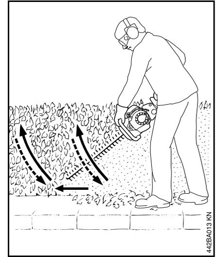
Swing the cutting blade from the bottom upwards in an arc – lower the nose of the blade, move along the hedge and then swing the blade up again in an arc.
