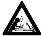
Kickback may occur when the moving saw chain near the upper quadrant of the bar nose contacts the wood or is pinched during limbing or when it is incorrectly used to begin a plunge or boring cut.
