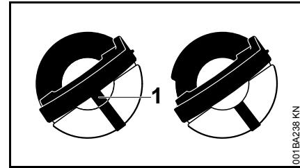
**Left:** Base of filler cap is rotated – interior marking (1) is aligned with the exterior marking.
