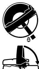
Fold the grip flush with the top of the cap. Grip the cap and check for tightness. If the grip does not lie completely flush with the cap and the detent on the grip does not fit in the corresponding recess in the filler opening, or if the cap is loose in the filler opening, the cap is not properly seated and tightened and you must repeat the above steps.
