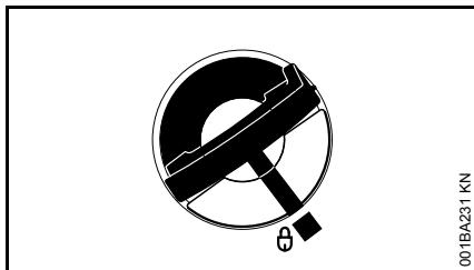
Then the markings on filler cap and housing will align.
