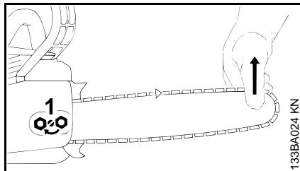
Retensioning during cutting work:
