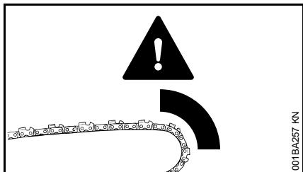
The powerful force used to cut wood can be reversed and work against the operator. If the rotating saw chain is suddenly and significantly slowed or
