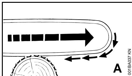
Pull-in occurs when the saw chain on the bottom of the bar is suddenly stopped when it is pinched, caught or encounters a foreign object in the wood. The reaction of the saw chain pulls the chain saw forward and may cause the operator to lose control.
