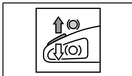
The activating mechanism for the STIHL Quickstop Plus chain brake system is integrated in the throttle trigger lockout (rear handle). One of the big advantages of this system is that the saw chain is automatically locked in position when carrying the running saw by the front handle (with the rear handle fully released).
