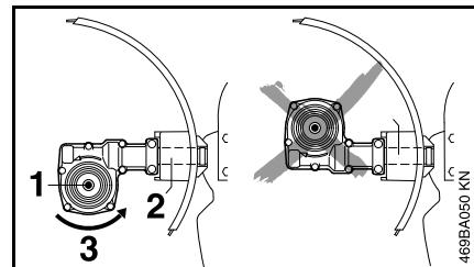
The axle (1) must be below the shaft (2). Direction of rotation (3) of MultiTool.
