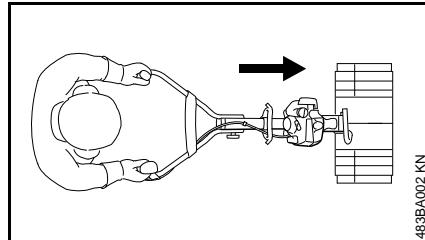
Operate the MultiEngine with MF-MM dethatcher in the forward direction only.
