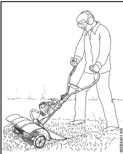
The MF-MM dethatcher MultiTool is designed to remove old, dried cuttings, moss, grass or root residue from lawns.
