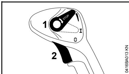
The throttle trigger (2) can be locked in any position.
