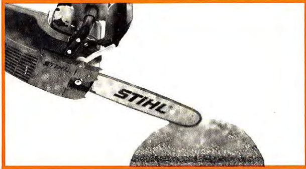
Checking chain lubrication
