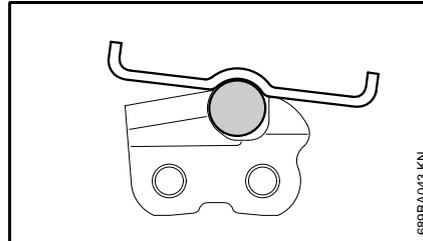
If the cutters are not the same length, they will have different heights. This makes the chain run roughly and can cause it to break.
