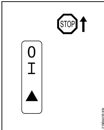
**Stop 0** – engine off – ignition is switched off
