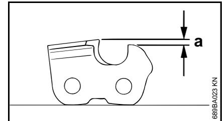
The depth gauge determines the height at which the cutter enters the wood and thus the thickness of the chip removed.
