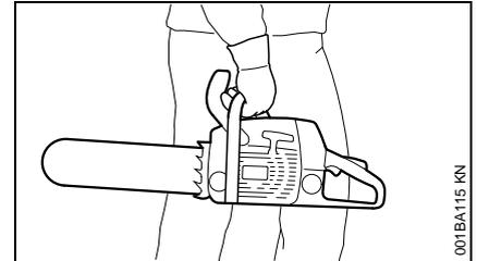
It may be carried only in a horizontal position. Grip the front handle in a manner that the machine is balanced horizontally. Keep the hot muffler away from your body and the cutting attachment behind you.
