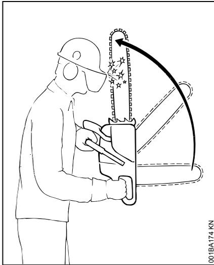
When a kickback occurs, the guide bar may rotate around the front handle. If the cutting position is such that the operator's left hand is gripping the front handle behind the hand guard, and if the left hand rotates around the front handle and makes a sufficiently forceful contact with the front hand guard, which is the Quickstop activating lever, this contact will activate a properly maintained Quickstop chain brake.
