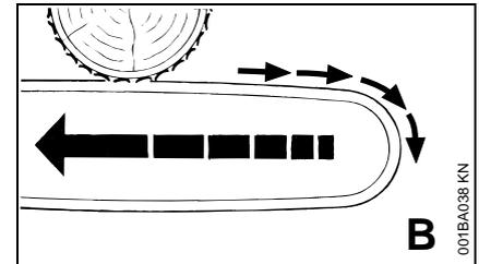
Pushback occurs when the chain on the top of the bar is suddenly stopped when it is pinched, caught or encounters a foreign object in the wood. The reaction of the chain may drive the saw rapidly straight back toward the operator and may cause loss of saw control. Pushback frequently occurs when the top of the bar is used for cutting.
