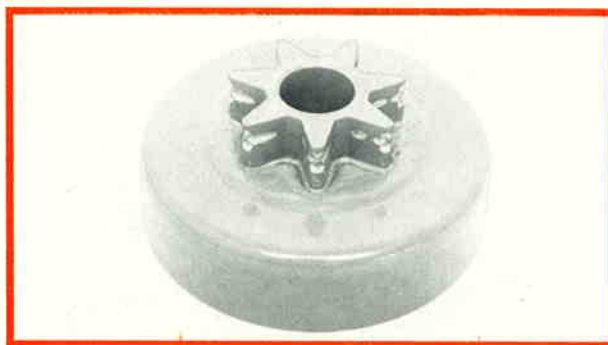
Worn chain sprocket
