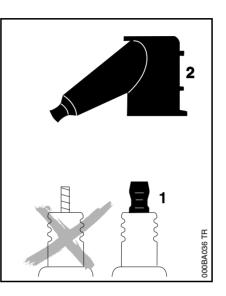
Fit a new spark plug after approx. 100 operating hours or earlier if the electrodes are badly eroded.
