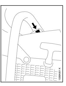
Press in the button (arrow) to open the decompression valve.
