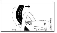
Pull the hand guard back toward the front handle: Co The chain brake is now disengaged your saw is ready for operation.
