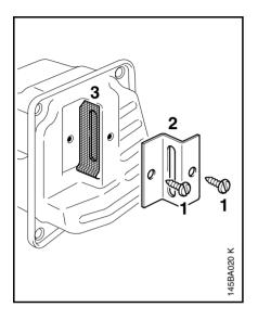
If engine is down on power, check the spark arresting screen in the muffler:
