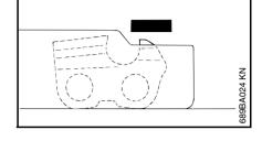
Round off depth gauges parallel to the stamped marking.
