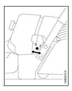
Switching on electric handle heating\*
