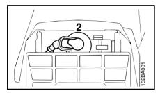
Pull the prefilter (1) upward and out -Pull off the spark plug boot (2) -
