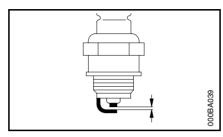
Use only resistor type spark plugs of the approved range.
