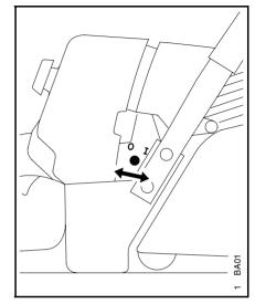
Switching on electric handle heating\*
