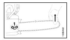
Retensioning during cutting work:
