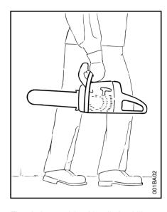
The chain guard (scabbard) should be over the chain and the guide bar, which should point backwards. When carrying your saw, the bar should be behind you.
