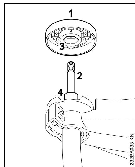
The thrust plate (1) is shipped with the DuroCut 5-2 and PolyCut 6-3. It is only required for these mowing heads.
