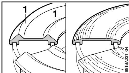
Do not continue using the mowing head if the raised moldings (1) on the base are missing or worn – see right illustration above. The mowing head may otherwise shatter and flying objects could result in injury to the operator or bystanders. Install a new mowing head.
