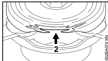
Do not continue using the PolyCut if one of the circular holes (1; arrow) becomes visible or if the projecting rim (2; arrow) has worn away. Install a new mowing head.
