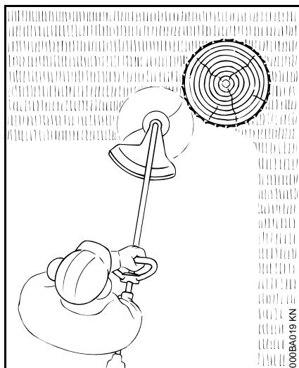
Mowing heads are to be used only on trimmers equipped with a line-limiting blade in the deflector in order to keep the line at the proper length (see "Main Parts" chapter in your instruction manual.)
